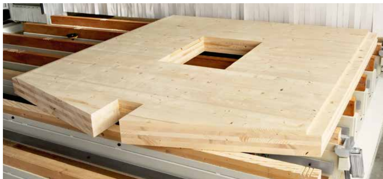
The structure of the worktable is anchored directly to the floor while the upper part is composed of material to be worked directly by the machine, in order to have a flat surface. It can be re-machined several times when surface gets scratched from use.
