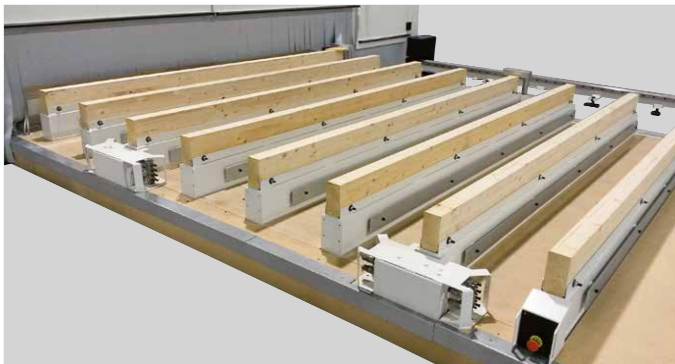
The machine design is based on a modular system allowing to customize the size of the worktable up to 50 m along the X-axis, to meet all production needs.
