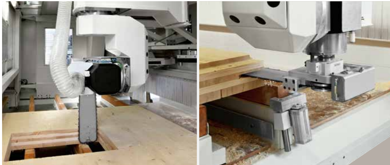
The aggregate "chainsaw" allows to quickly realize: 90° openings, cutting with nesting technology, deep grooves and slots on all sides of the element.
