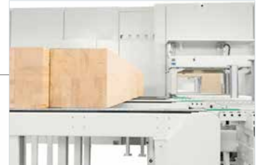
Handling of large elements with the possibility of positioning workpieces up to 500 mm thick on the loading chains.
