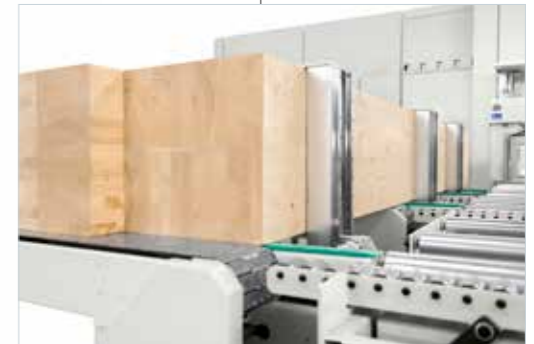
Precision and safety during loading thanks to NC-controlled clamps that ensure a perfect grip.
