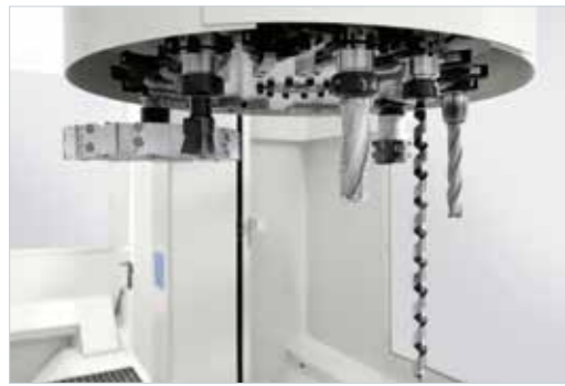
Reduced tool change time thanks to the strategic location of the Rapid 15 tool store, which can accommodate up to 16 tools including aggregates.
