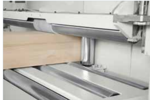
No vibrations thanks to the use of pressure rollers that lock the element during machining.
