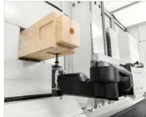
6-axis machining head unit for maximum manufacturing flexibility.
