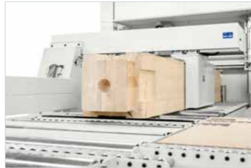
Firm and precise movement of the element by means of large self-centering clamps.
